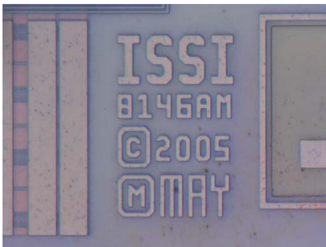
Decapsulation sample D/C:2231:ISSI 8146AM 2005 MAY
