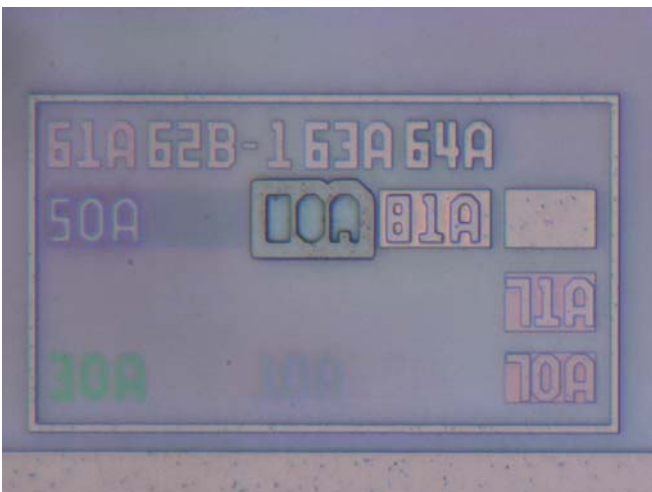
Decapsulation sample D/C:2231:Die marking
