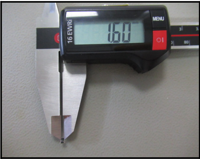
Dimension Measurement E1=1.60 mm, (Pass)
