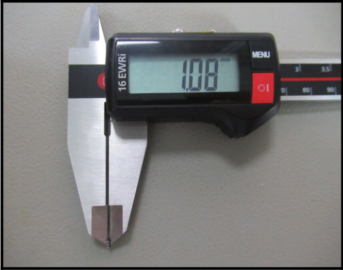
Dimension Measurement A2=1.08 mm, (Pass)
