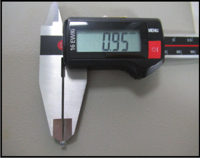
Dimension Measurement e=0.95 mm
