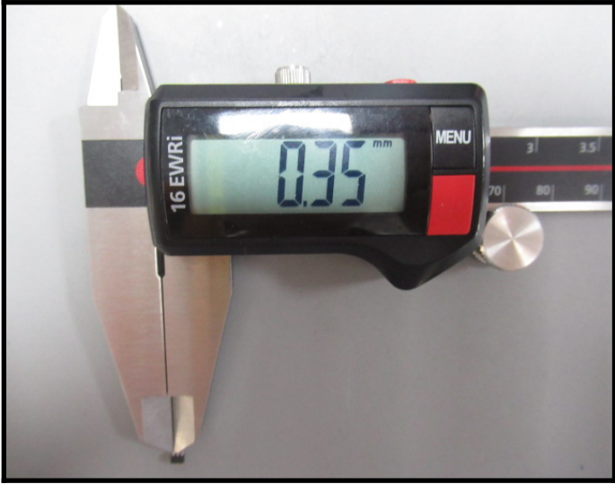
Dimension Measurement b=0.35 mm, (Pass)
