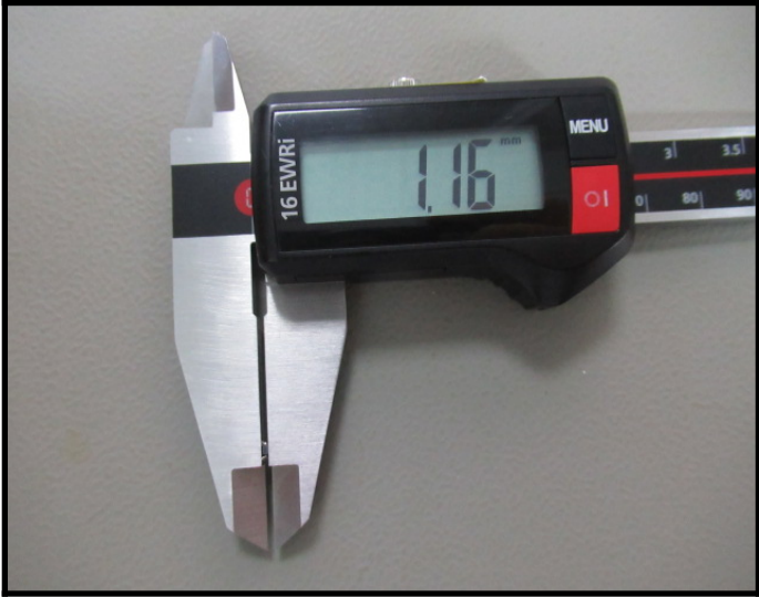
Dimension Measurement A=1.16 mm, (Pass)
