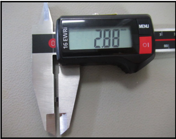
Dimension Measurement E=2.88mm, (Pass)
